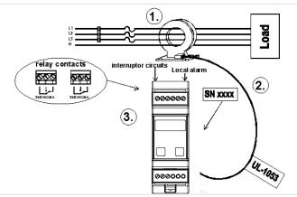
Ground fault protection can be used for equipment protection only - not for personal protection.
