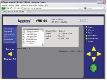
The list of the latest alarms and equipment faults can be viewed on the web interface. It is also possible to change the basic settings of the VRE device and restore some or all settings to the factory default values. Also username and passwords can be modified on the web interface.
