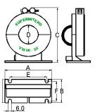
In custom made models, please give length and height information. Maximum and minimum measures of custom made busbar transformers (window type) are: min H 50mm max H 204mm min L 50mm max L 660mm
