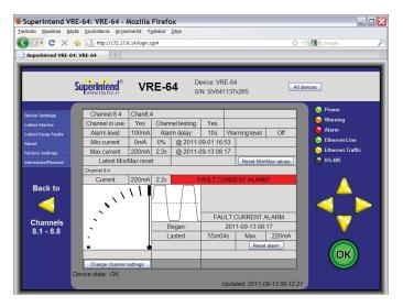
Some detailed information of one channel is shown on the channelspecific view. In addition to the momentary fault current level, the channel view shows the fault current waveform, alarm status of the channel and minimum/maximum fault current history. Channel settings are shown and it is also possible to change them.
